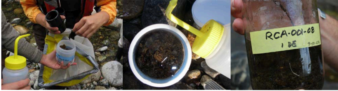
CABIN kick net collection of benthic invertebrates, and transfer of benthic sample into a jar for later identification.
